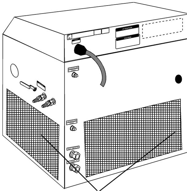
The pump motor overload protector is located directly under the fluid reservoir. It is in the left rear corner for HX200s and HX300s units. It is at the side access panel for HX500s and HX750s units.
