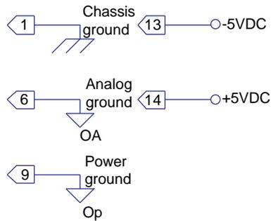
Access Receptacle Equivalent circuits
