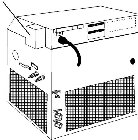
With the ENABLE/DISABLE switch set to ENABLE, the heater will cycle on and off under the control of the temperature controller. With the switch in the DISABLE position, the heater will remain off.
