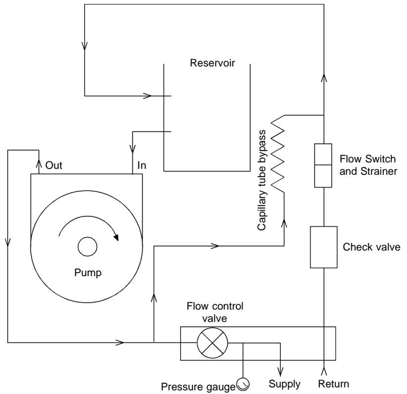
**Pump Flow Diagram (PD and TU Pumps)**
