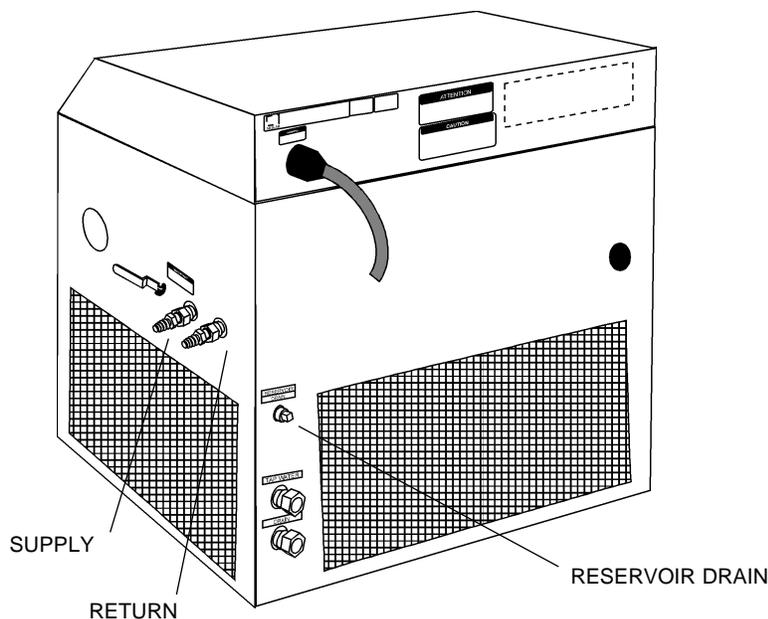
Two plumbing adapters ( $\frac{3}{4}$  inch MPT x  $\frac{5}{8}$  inch hose) are included with the unit. If the unit is being plumbed to the instrument being cooled using flexible tubing, install the adapters in the SUPPLY and RETURN plumbing ports. To prevent leaking, wrap the threads of the adapters with Teflon® sealing tape before installing them in the plumbing ports. The adapters will accept  $\frac{1}{2}$  or  $\frac{5}{8}$  inch ID flexible tubing.
