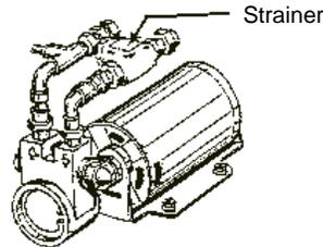
Before cleaning the strainer, disconnect the line cord from the power source and drain the reservoir.
