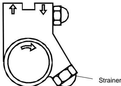
PD-2 Pump: a wire mesh screen is located under the large hex nut on the pump suction line.
