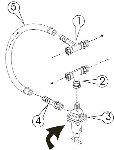
The EPR is now installed. Connect the inlet (to your application) to the remaining fitting of the Outlet Tee Assembly (2). Connect the outlet (from your application) to the remaining fitting of the Inlet Tee Assembly (1).
